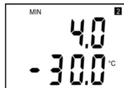
Press button again to display range and type of value for output 2 (symbol „2“). Here it is ambient temperature („°C“), when 4 mA corresponds to -30 °C.
