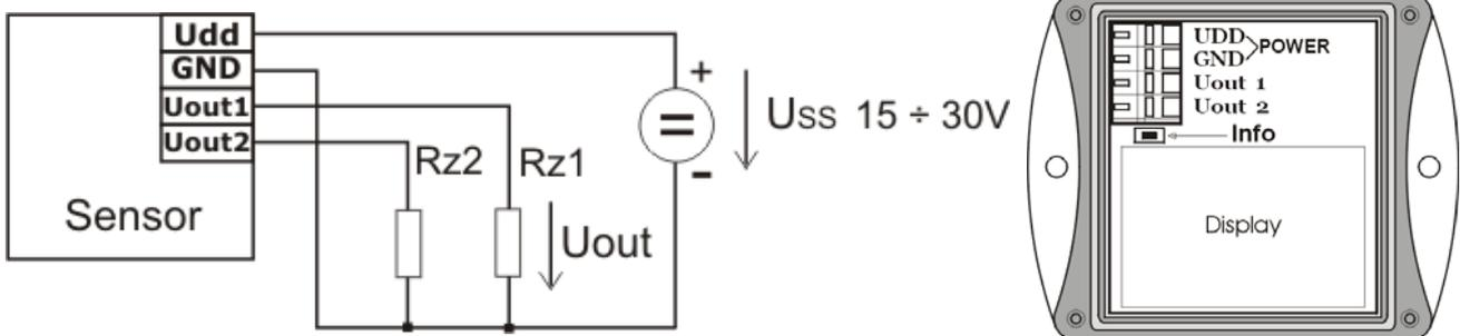
Maximum load current of each voltage output is 0.5 mA
