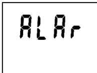
Pressing the ENTER key enables to enter the mode of setting alarm limits for all quantities (see below).
