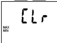
Clearing of minimum and maximum memory of all values. Memory is cleared after pressing ENTER key. Clearing is confirmed by reading YES on the LCD lower display.
