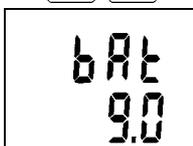
Battery voltage of partially loaded battery is displayed. This value illustrates battery condition.
