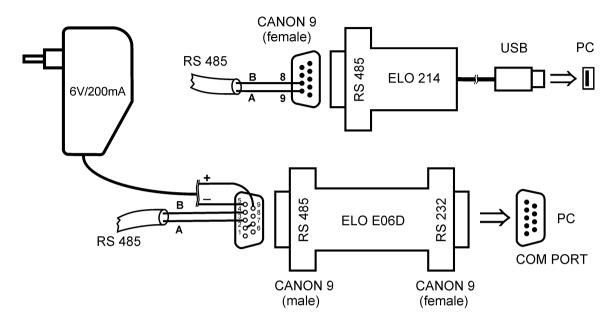
The ELO E06D converter is an optional accessory for connection of transmitter with RS485 interface to the PC via serial port RS232. Connect connector marked RS232 directly to the PC, connect power to connector marked RS485. Power voltage +6V DC from an external acdc adapter connect to pin 9, 0V connect to pin 5. Also mutually connect pin 2 and pin 7. Link RS485 is connected across pin 3 (A+) and pin 4 (B-).
