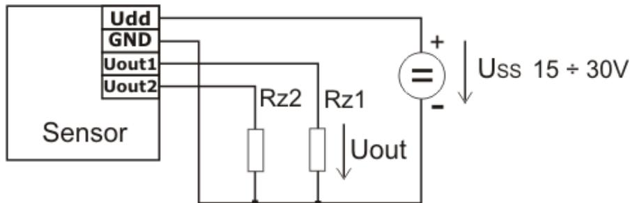
Maximum load current of each voltage output is 0.5 mA.
