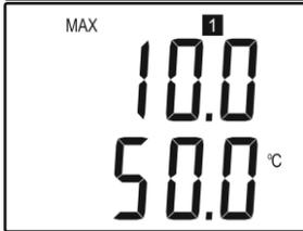
Next button press shows values for upper scale limit. (the same channel, the same value) by the same rules as at previous case. Here 10 V corresponds with temperature of 50 °C.
