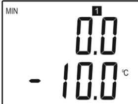
Short button press shows low range and type of measured value for first output (output Uout1, at LCD indicated by symbol „1“). Type of measured value is indicated with appropriated value unit. (here °C = temperature). Upper line shows voltage value which is assigned to value of measured value (lower display line). Here 0 V corresponds with temperature of -10 °C.
