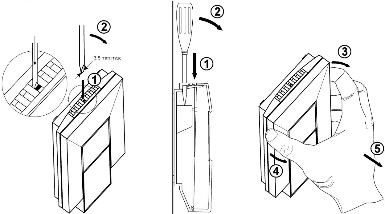
Figure2: Device demounting
