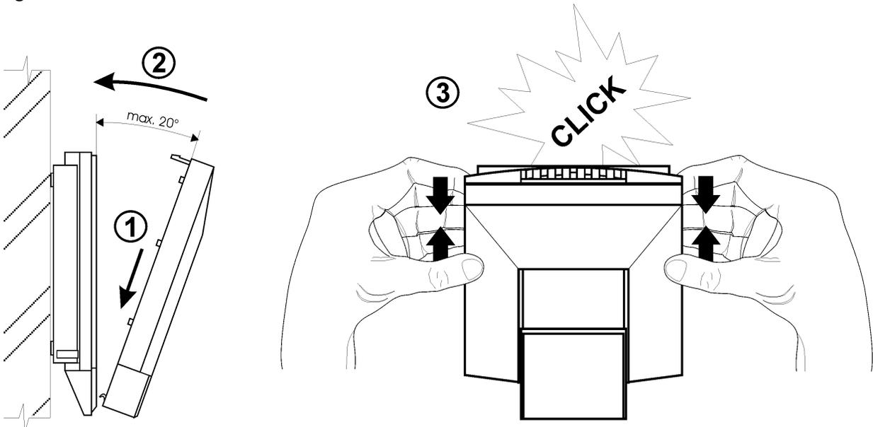
Figure1: Device mounting
